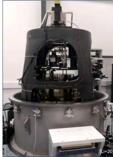
Planck Waage (TU Ilmenau / PTB)
