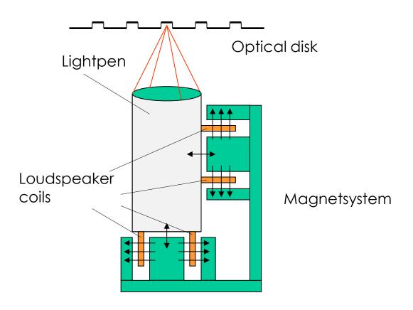
Sensing of position error between light spot & compact disc track:
