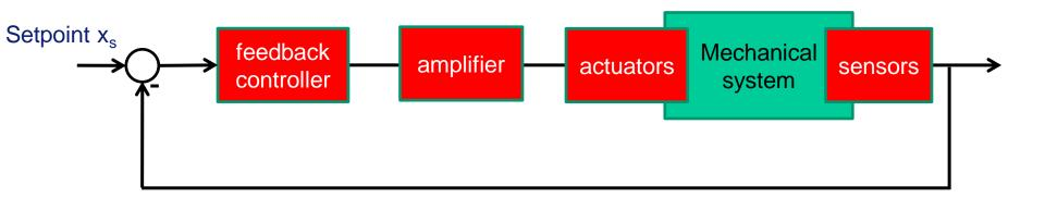
An error is required to generate a servo force.
