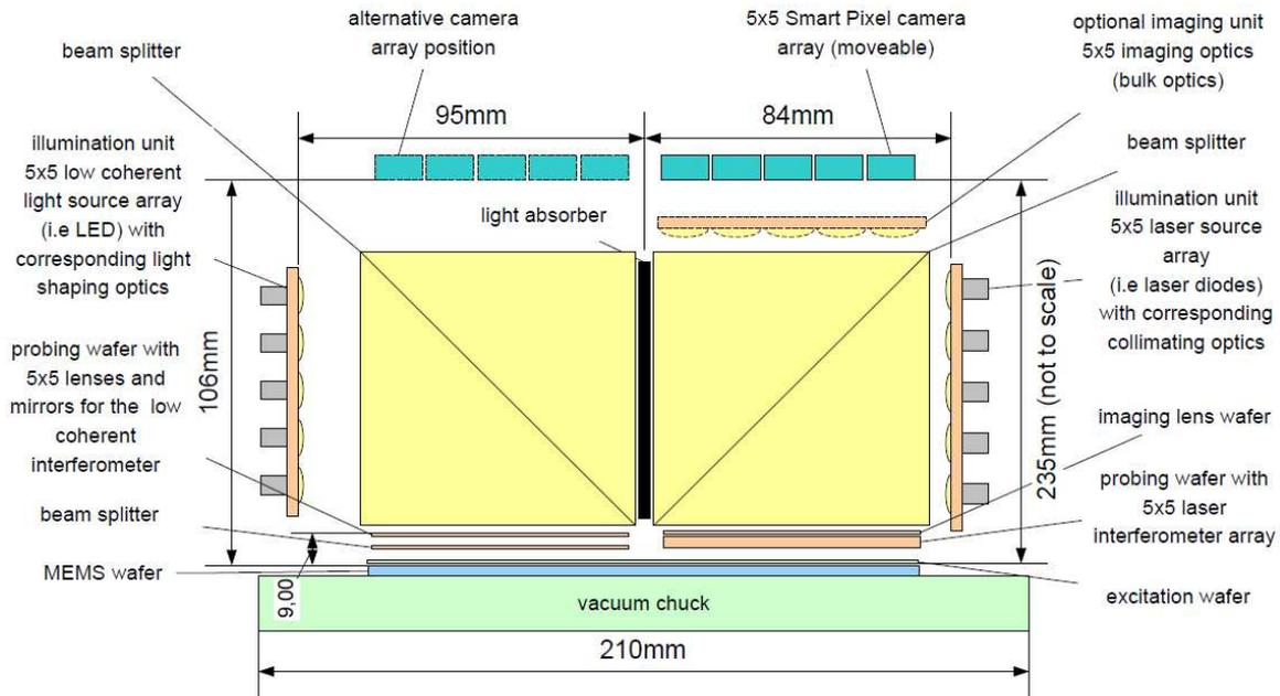
Figure 1: SMARTIEHS instrument configuration: Side view with dimensions.
