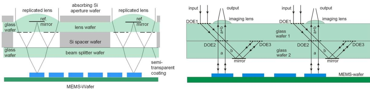
a) low coherent Mirau interferometer
